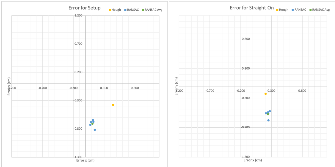
Figure 7: Black ball position error
